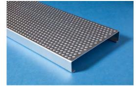
treads possess end caps (with slots and mounting holes) and margins on every side. Tread-Grip<sup>®</sup> grating is available in different gauges (depending on the product) with HRP & O or pre-galvanized steel options, as well as .125" 5052-H32 aluminum.
